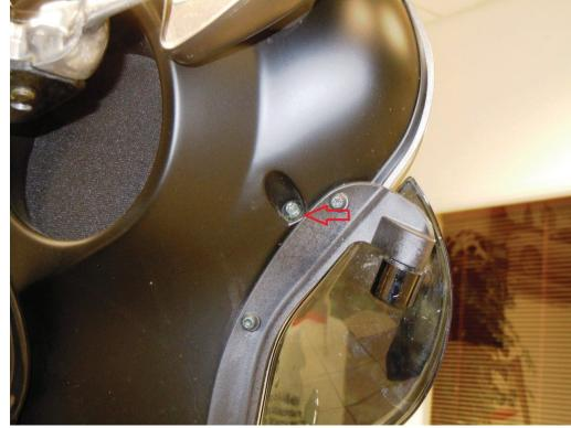
2. Locate and remove the two bolts on the upper faring one on each side
