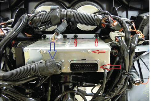
7. On the 23 Pin connector show above with a Blue arrow Connect the Red wire using the supplied t tap to pin 20 on the main radio plug Connect the Black wire using the supplied t tap to pin 19
